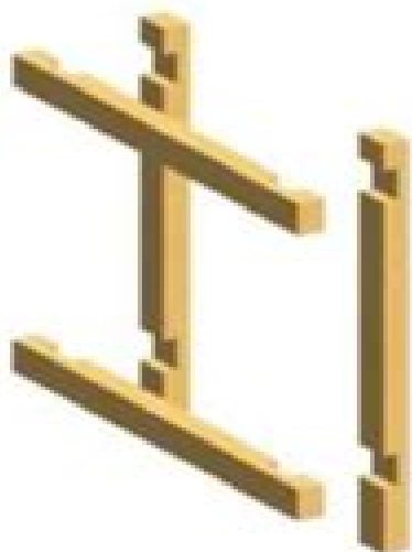
Figure 3. Detail of Cross Halving Joint for pombalino buildings [18]
