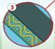
These loose electrons are now free to move, creating an electric current from the positive and negative charges now present. They pass through the layers of the solar cell.
