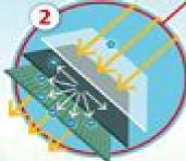
Photons hit the solar panel, knocking electrons free of the silicon atoms within the solar cells.
