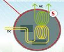
The inverter converts the direct current (DC) to alternating current (AC), which is what is used to provide power.
